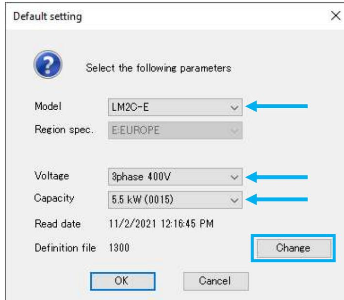
Figure 8. Configuration box from FRENIC-Loader 4
